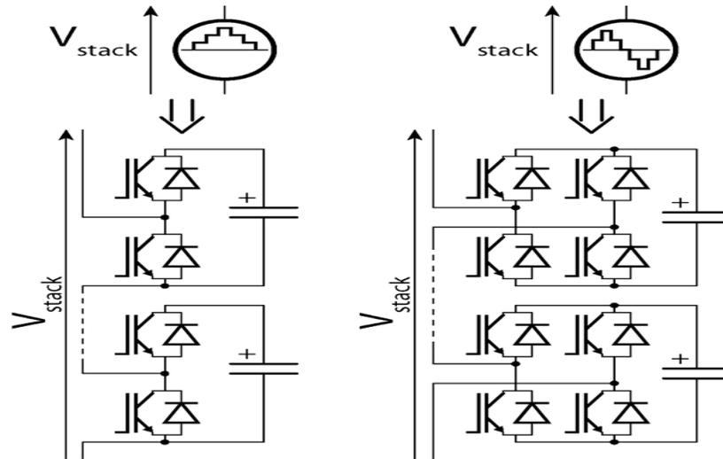
Figure 1: Schematic of half-bridge cells (left) and H- Bridge cells (right)
