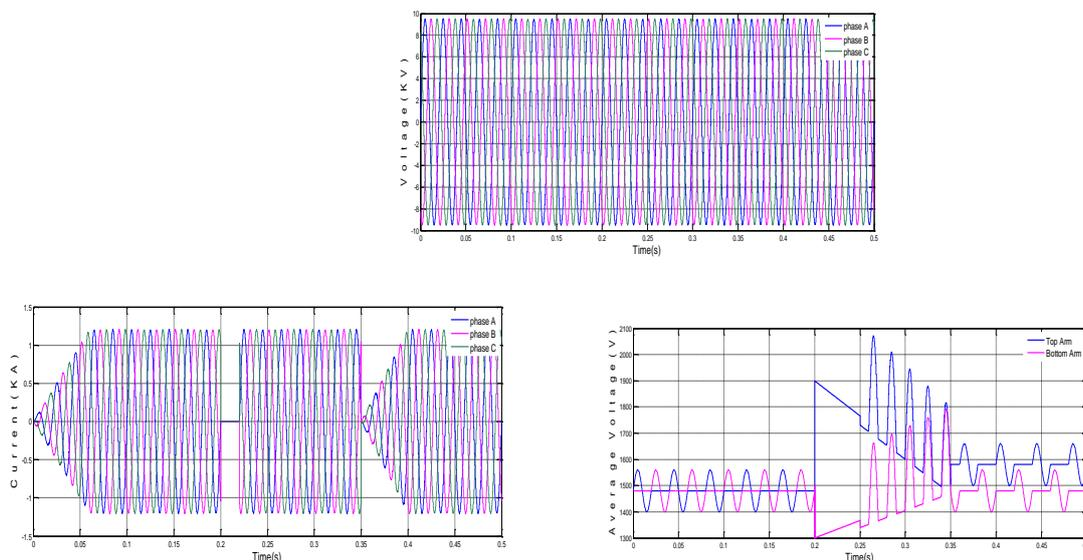
**Figure: 6** Simulation results of a proposed model running in rectifier mode when a dc-side fault occurs between 0.20 and 0.35 s.
