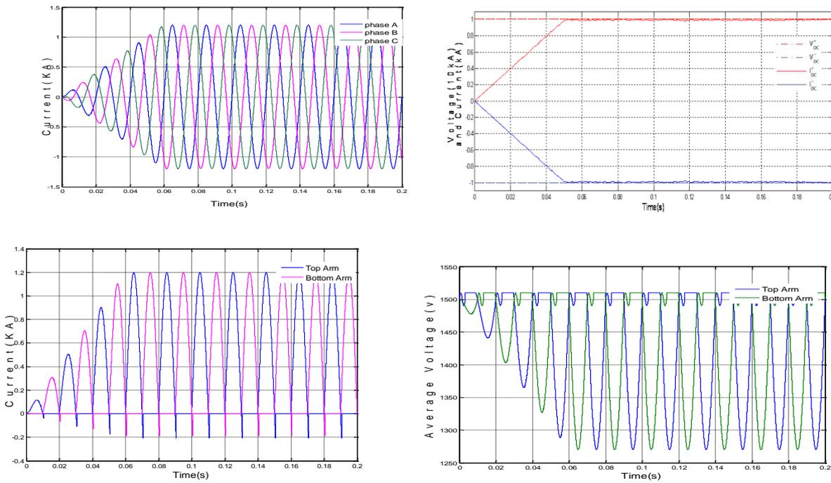
**Figure: 4** Simulation results of a proposed model running in rectifier mode under normal conditions.
