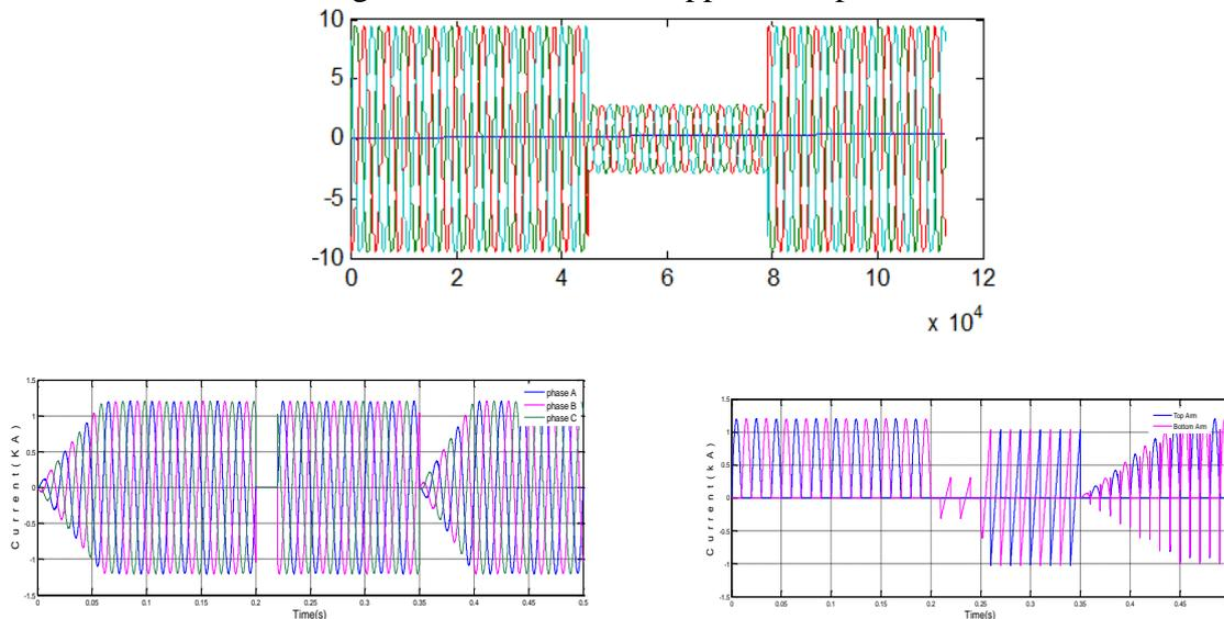
**Figure: 5** Simulation results of a 20-MW AAC model running in rectifier mode when an ac-side fault occurs between 0.20 and 0.35 s.
