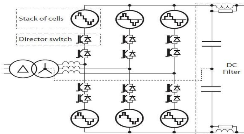
**Figure: 3** Schematic of the cascaded H-bridge and arm converter, with the optional middle-point connection shown in a dashed line.
