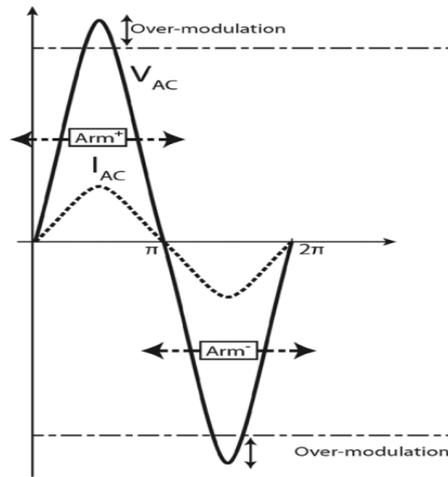
**Figure 2:** Idealized voltage and current wave Waveforms over one cycle in a phase
